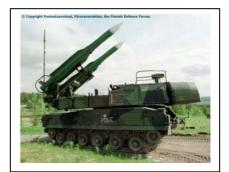
Power Plant = solid-rocket Speed = Mach 3.5 Range = 1.6-15nm Ceiling = 45000ft Lethal Radius = 55ft
